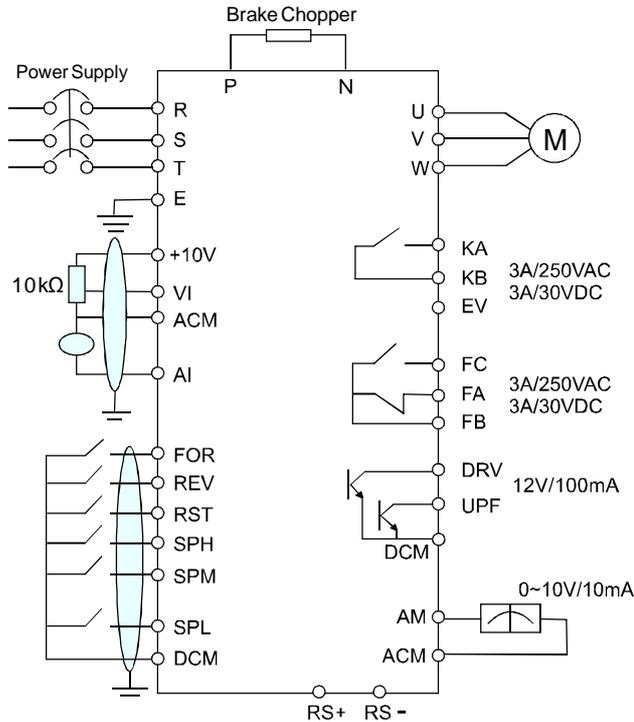
The wiring diagram of expansion board:
