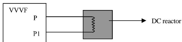
Note: Connecting point reserved on 37W HLP frequency converter; no connection is allowed for those below 37W.
